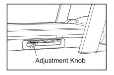
trolled with the knob on the right side of the treadmill. To increase the firmness, turn the knob clockwise; to decrease the firmness, turn the knob counterclockwise. Note: The faster you run on the treadmill, or the heavier your weight, the firmer the cushioning system should be. If the cushioning system is too soft, you will hear the walking platform hitting the platform bumpers as you run.
